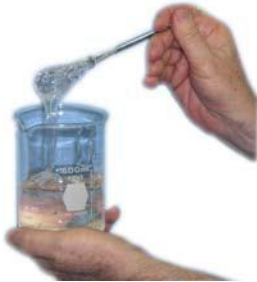
PSF-10,000cSt Pure Silicone Fluid is a high viscosity polydimethylsiloxane that meets federal spec VV-D-1078 "Silicone as Damping Fluid".
